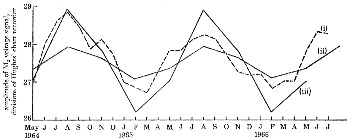
FIGURE 12. Effect on the signal of seasonal variation of Cemaes Bay-Castletown cable. (i) Hughes's observations. (ii) From theoretical model, \sigma_E = 0.015 \text{ S m}^{-1} . (iii) From theoretical model, \sigma_E = 0.0225 \text{ S m}^{-1} .
